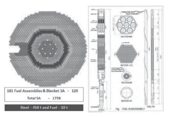
FIGURE 7. PFBR 500 Core With 181 MOX Fuel Assemblies In Centre Surrounded By 120 RDU Oxide Blanket Assemblies
